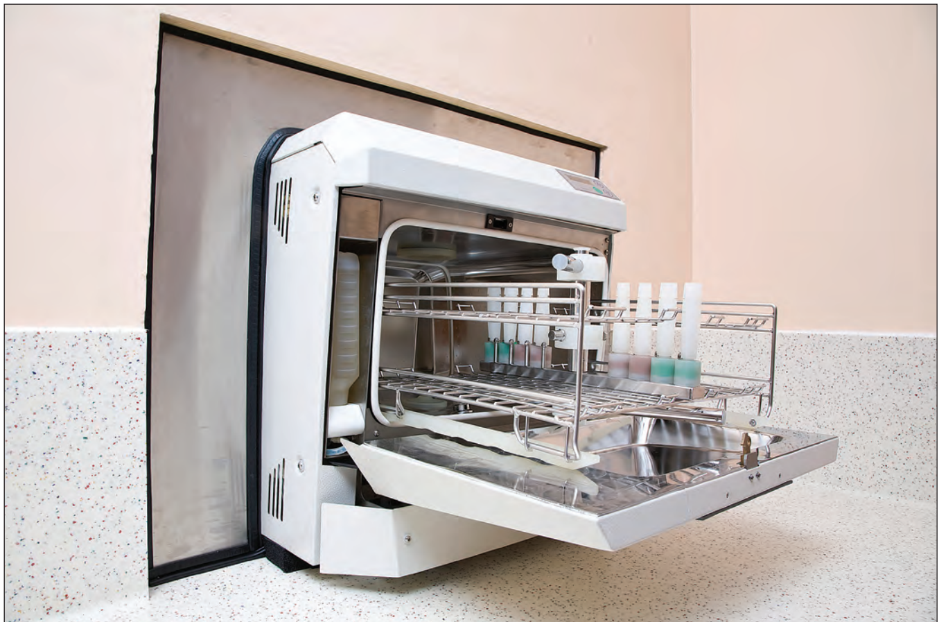
Using a washer-disinfector is the preferred method for cleaning dental instruments because it offers the best option for the control and reproducibility of cleaning
